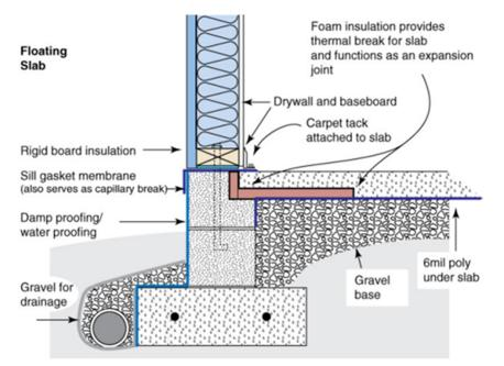
Figure 3: Slab and stem wall configuration
