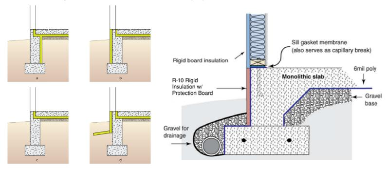
Figure 1: Common slab edge insulation locations<sup>3</sup>
